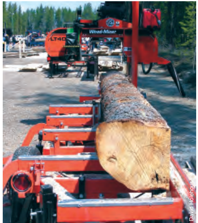
Portable sawmills, like the Wood-Mizer line from Salmon Arm, help landowners turn beetle-killed and other timber into products with value
